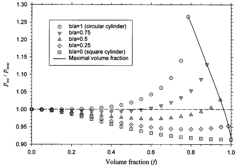
Fig. 5. Ratio of electric dipole moments in the direction of  $E^{\text{inc}}$  with mutual coupling ( $p_{\text{wc}}$ ) and without mutual coupling ( $p_{\text{woc}}$ ) included between particles. The incident field has  $E^{\text{inc}} = 1$  V/m and  $\phi^{\text{inc}} = 90^\circ$ .
