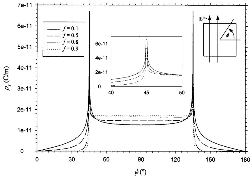
Fig. 4. Surface charge distribution on square conducting cylinders for various volume fraction  $f$  ranging from 0.1 to 0.9. The incident field has  $E^{\text{inc}} = 1$  V/m and  $\phi^{\text{inc}} = 90^\circ$ .
