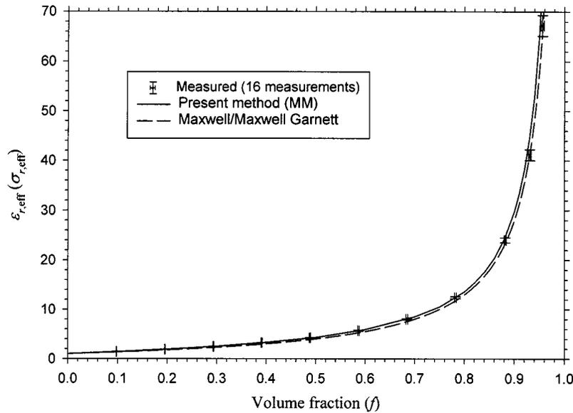
Fig. 8. Predicted quasi-static effective permittivity and measured effective conductivity for a simple cubic lattice of conducting cubes. The measurements were performed at 80 kHz. Error bars indicate one standard deviation in both  $\sigma_{r,eff}$  and volume fraction.
