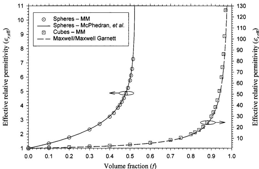
Fig. 3. Computed  $\epsilon_{r, \text{eff}}$  for 3-D lattices of conducting spheres and conducting cubes. Our MM solution for conducting spheres is compared with data from [10]. Note that the vertical  $\epsilon_{r, \text{eff}}$  scales for the sphere and cube data are much different.
