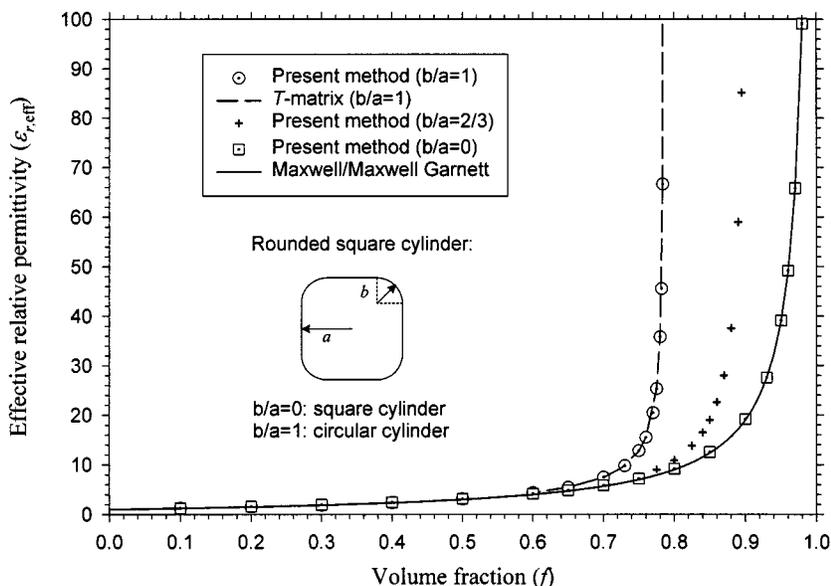
Fig. 2. Computed  $\epsilon_{r, \text{eff}}$  for three 2-D conducting particle shapes (circle, rounded square, and square cylinders). Also shown are the  $T$ -matrix results for circular conducting cylinders [9]. The Maxwell/Maxwell Garnett (MG) results indicate the lower bound for the static permittivity of these three composite materials.
