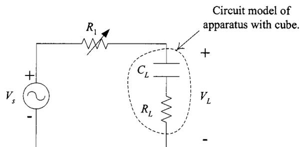
Fig. 7. Equivalent quasi-static circuit model for the experimental measurements of  $\sigma_{r,eff}$  using the apparatus in Fig. 6. The effects of the brass plates, brass cube, and Lexan box are modeled by the series combination of  $C_L$  and  $R_L$ .
