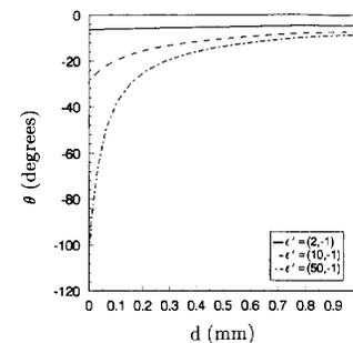
Fig. 9. Phase of the reflection coefficient in degrees as a function of lift-off for various permittivities of a slab occupying the lower half space. Frequency is 1 GHz,  $b = 14$  mm,  $a = 6.08$  mm,  $\epsilon_{Rc}^* = 2.54$ , and six  $TM_{0n}$  modes were used.
