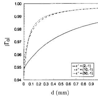
Fig. 8. Magnitude of the reflection coefficient as a function of lift-off for various permittivities of a slab occupying the lower half space. Frequency is 1 GHz,  $b = 35$  mm,  $b/a = 2.3$ , and six  $TM_{0n}$  modes were used.
