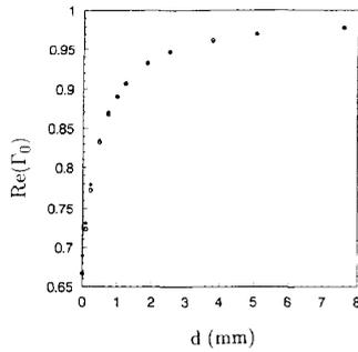
Fig. 10. The real part of the reflection coefficient as a function of lift-off compared with theory,  $\epsilon_{RC}^* = 2.54$ ,  $\epsilon_{RS}^* = (6.15, -0.029)$ , and six  $TM_{0n}$  modes were used. The  $\circ$  denotes experimental values. The combined standard uncertainty at zero lift-off due to the uncertainty in lift-off is  $u_c = 0.045$ .
