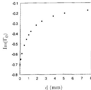
Fig. 11. The imaginary part of the reflection coefficient as a function of lift-off compared with theory,  $\epsilon_{RC}^* = 2.54$ ,  $\epsilon_{RS}^* = (6.15, -0.029)$ , and six  $TM_{0n}$  modes were used. The  $\circ$  denote experimental values. The combined standard uncertainty at zero lift-off due to the uncertainty in lift-off is  $u_c = 0.045$ .
