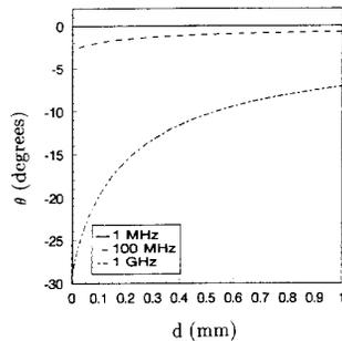
Fig. 5. The phase of the reflection coefficient in degrees as a function of lift-off for various frequencies of a slab occupying the lower half space. The simulation uses  $b = 14$  mm and  $a = 6.08$  mm with  $\epsilon_{Rc}^* = 2.54$ ,  $\epsilon_{Rs}^* = (10, -1)$ , and six  $TM_{0n}$  modes were used.
