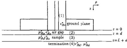
Fig. 1. The open-ended coaxial probe over a sample with an air gap between sample and probe. The cases considered are (1) semi-infinite media, (2) short-circuit termination location at  $z = d + L$ , and (3) material termination where a well-characterized material occupies the region starting at  $z = d + L$  and extending to  $\infty$ .
