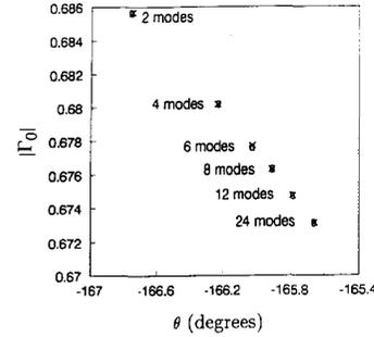
Fig. 3. The magnitude of the reflection coefficient for  $d = 0$  versus phase at 1 GHz for  $a = 2.333$  mm and  $b = 7.549$  mm,  $\epsilon_{Rc}^* = 2.15$ , with  $\epsilon_{Rs}^* = (100, -100)$  where  $x$  denotes current paper results and  $0$  denotes Hodgetts' results.
