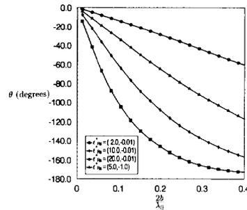
Fig. 7. The phase in degrees as a function of coaxial line outer conductor radius, normalized to wavelength in air, of a slab of varying dielectric parameters occupying the lower half space. The computation uses  $b = 35$  mm and  $b/a = 2.3$ , zero lift-off, and six  $TM_{0n}$  modes were used.
