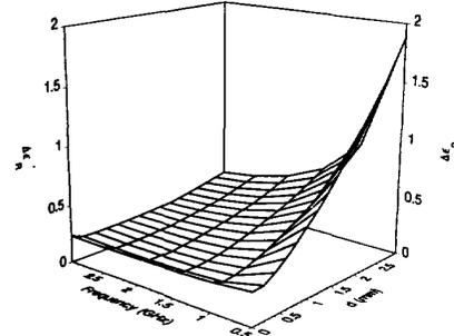
Fig. 2. Two-dimensional plot of the combined uncertainty in  $\epsilon_{Rs}'$ . The parameters used were  $\epsilon_{Rs}^* = (10, -0.1)$ , six  $TM_{0n}$  modes,  $\Delta d = 0.000254$  m,  $\Delta\theta = 0.5^\circ$ ,  $\Delta|\Gamma_0| = 0.002$ .
