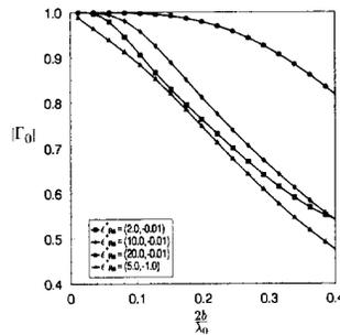
Fig. 6. The magnitude of the reflection coefficient as a function of coaxial line outer conductor radius, normalized to wavelength in air, of a slab of varying dielectric parameters occupying the lower half space. The computation uses  $b = 14$  mm and  $a = 6.08$  mm with  $\epsilon_{Rc}^* = 2.54$ ,  $\epsilon_{Rs}^* = (10, -1)$ , zero lift-off, and six  $TM_{0n}$  modes were used.
