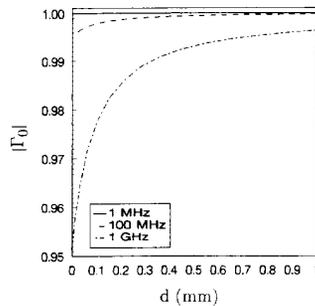
Fig. 4. The magnitude of the reflection coefficient as a function of lift-off for various frequencies of a slab occupying the lower half space. The probe is assumed to have  $b = 14$  mm and  $a = 6.08$  mm with  $\epsilon_{Rc}^* = 2.54$ ,  $\epsilon_{Rs}^* = (10, -1)$ , and six  $TM_{0n}$  modes were used.
