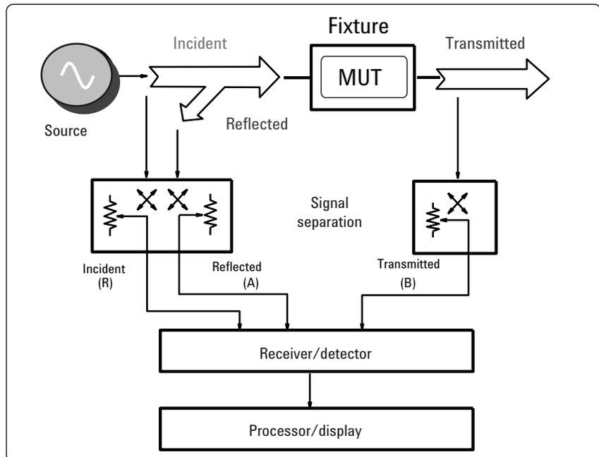
**Figure 11. Network analyzer**
