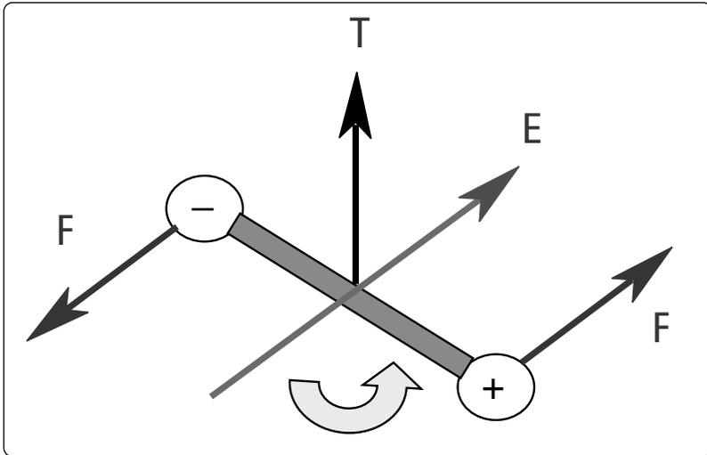
Figure 8. Dipole rotation in electric field
