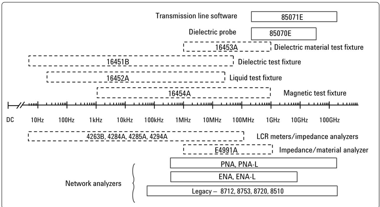
Figure 26. Agilent Technologies instruments and fixtures
