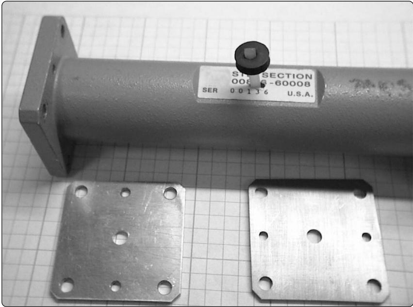
**Figure 23. X-band cavity resonator parts and inserted sample**
