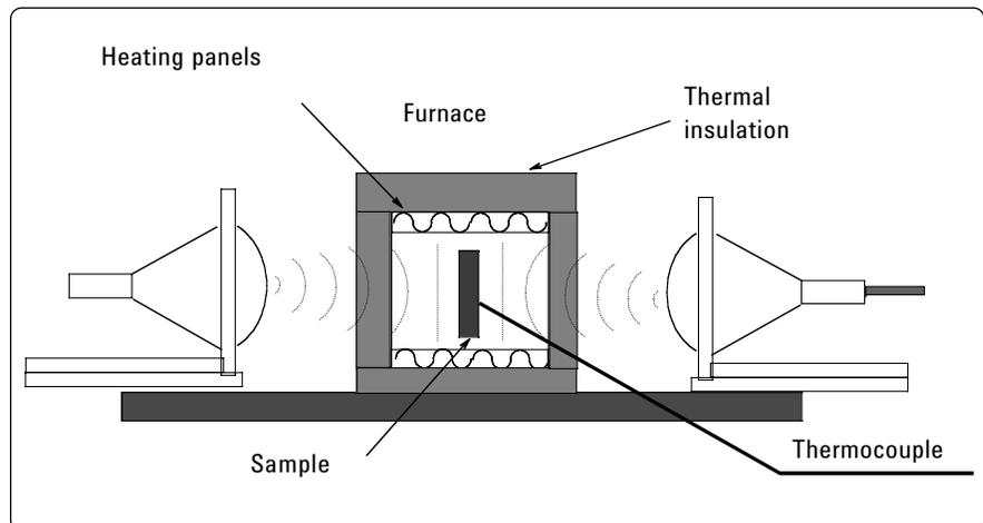
**Figure 21. High temperature measurement in free space**
