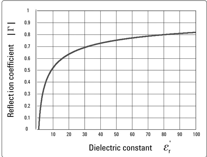
Figure 6. Reflection coefficient versus dielectric constant
