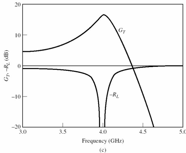
The **desired gain of 16.7 dB was attained** at 4 GHz with a good match at port 1. The response is narrowband because the transistor is not well matched to  $50 \Omega$  since  $|S_{11}| \approx 0.6 - 0.8$  and  $|S_{22}| \approx 0.7 - 0.8$ . However, bandwidth was not a consideration in this design. We designed for maximum gain at a specified frequency.
