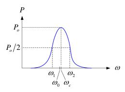
Notice that  $\omega_0$  is **not** the center frequency  $\omega_c$ . The text defines
