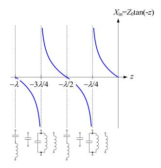
So, one could use a  $\lambda/4$ -long short circuit stub to act as the shunt parallel resonant circuit for the bandpass filter.
