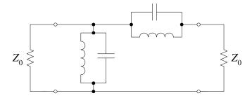
This is the bandpass filter topology are searching for! It has been obtained very easily using stub resonators and TL impedance inverters.
