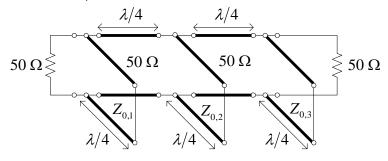
The required characteristic impedances of these stubs can be expressed in terms of the prototype filter coefficients,  $g_k$ , as given by equation (8.131):
