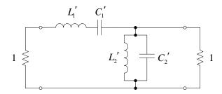
We could use the first Kuroda identity to transform  $L_1'$  to a shunt capacitance, but what about the series capacitance  $C_1'$ ?
