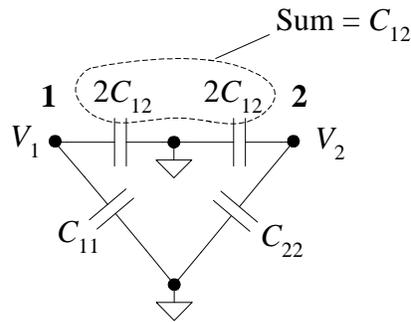
The effective capacitance to ground of either conductor in this configuration is then
