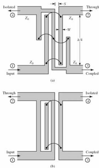
This is one method for obtaining **higher coupling coefficients** (up to approximately 2-3 dB or so) than what is possible with regular coupled line directional couplers.
