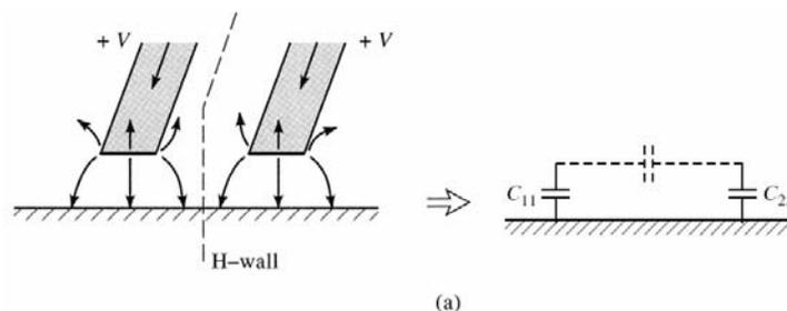
Hence, the electric field has **even symmetry** about the plane of symmetry (POS). This plane is called an “**H-wall**.”
