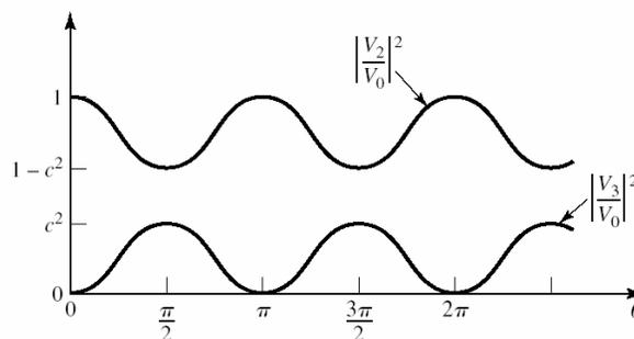
Notice from these plots that we can **maximize**  $|V_3/V|^2$  and **simultaneously minimize**  $|V_2/V|^2$  when  $\theta = \pi/2, 3\pi/2, \dots$  so that  $l = \lambda/4, 3\lambda/4, \dots$ . In these cases, (11)-(14) become
