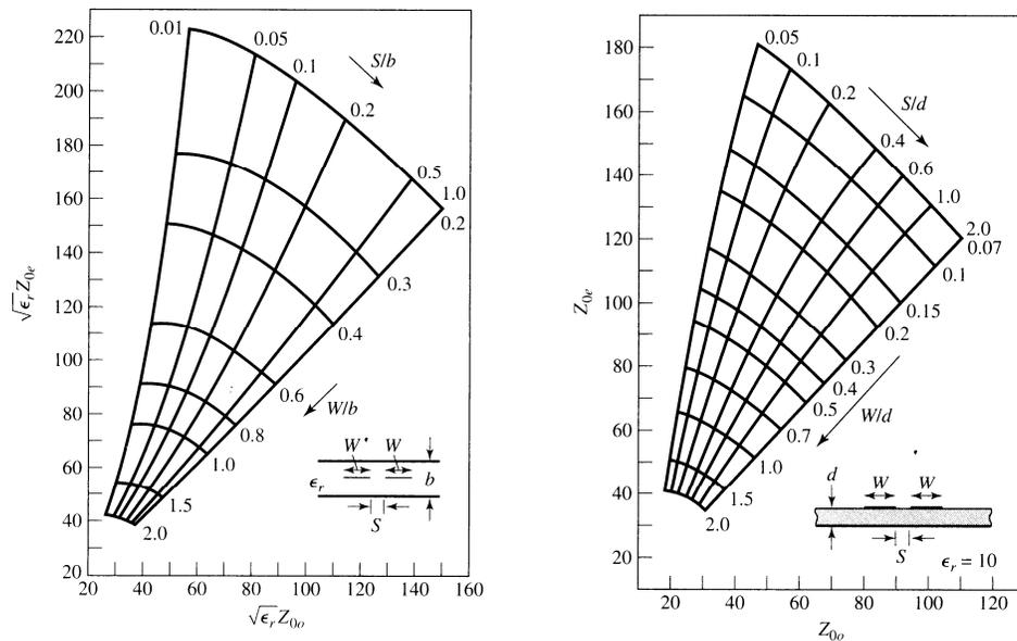
Recall that striplines support pure TEM modes, while microstrips do not. To use the stripline design curves, **scale** the even and odd mode impedances upward by  $\sqrt{\epsilon_r}$ , while the microstrip design curves apply **only for  $\epsilon_r = 10$** .
