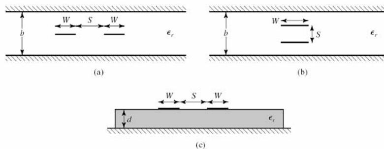
This can be a **serious problem** on PCBs where lands are close together and carry signals changing rapidly with time. EMC engineers face this situation in high speed digital circuits and in multiconductor TLs.
