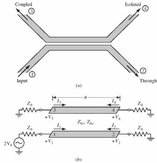
As mentioned earlier, we will apply an even-odd mode analysis for this coupler. Recall that in order to add these two solutions, both problems must have the same boundary conditions. That's why we terminate the TLs with  $Z_0$  rather than  $Z_{0,e}$  or  $Z_{0,o}$ .
