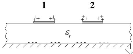
When voltages are applied, charge distributions will be induced on all of the conductors. The voltages and total charges are related to each other through **capacitance coefficients**  $C_{ij}$ :
