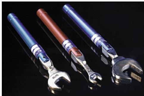
If you over-tighten a connection, it is possible you will damage the VNA connector, the cable, or your microwave circuit. There may be different types of torque wrenches lying about the lab. Be certain you are using the **BLACK**-handled torque wrench.
