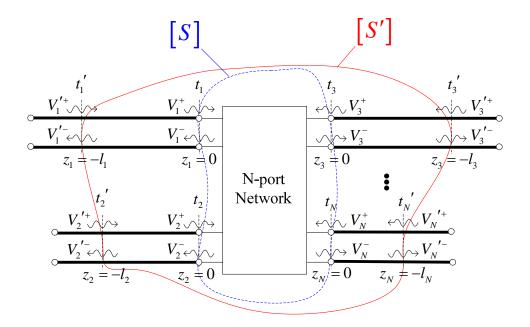
To be specific, let S be the scattering matrix of a network with reference planes (i.e., ports) at  $t_n$ , while [S'] is the scattering matrix of the network with the reference planes shifted to  $t_n'$ .
