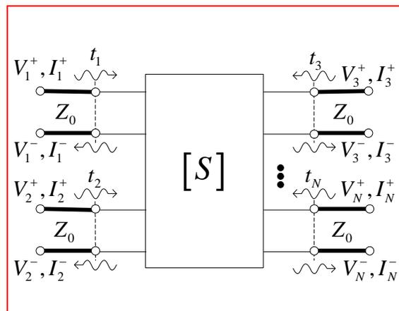
Rather than focusing on the *total* voltages and currents (i.e., the sum of “+” and “-” waves) at the terminal planes  $t_1, \dots, t_n$ , the  **$S$  parameters** are formed from ratios of reflected and incident voltage wave amplitudes.
