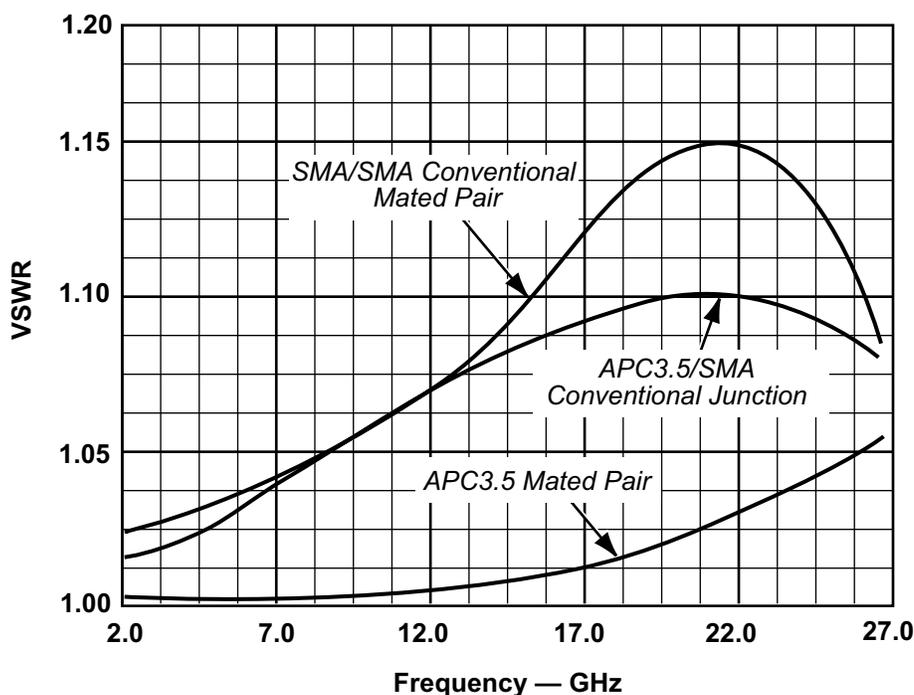
**Figure 4:** Complementary matching occurs when an APC3.5 connector mates to a "conventional" male or female SMA. The matching allows the APC3.5 to SMA junction to surpass the performance of the SMA mated pair. These results indicate that the APC3.5 can be used to improve SMA measurements.
