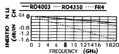
▲ Fig. 4 The insertion loss vs. frequency.
