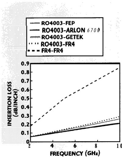
▲ Fig. 6 RO4003 50  $\Omega$  stripline insertion loss.
