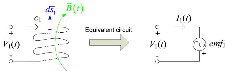
Given the direction for  $\vec{B}$  and the assumed direction for  $c_1$  (which gives rise to the direction of  $d\vec{s}_1$ ), then from the equivalent circuit and (4) we find
