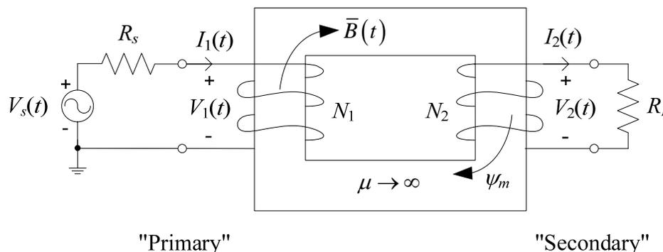
Notice that there is **no continuous path** for conduction current from the voltage source  $V_s$  to the load resistor  $R_L$ . These two ports instead are electrically “**coupled**” to each other indirectly by the principal of **induction** from Faraday’s law.
