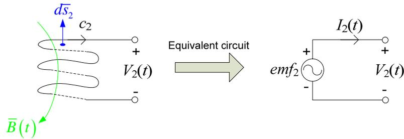
Notice here that the direction of  $d\bar{s}_2$  (dictated by the given direction for  $I_2$  and hence  $c_2$ ) is opposite that of  $\bar{B}$ . Consequently, from the equivalent circuit and using (4) again we determine that
