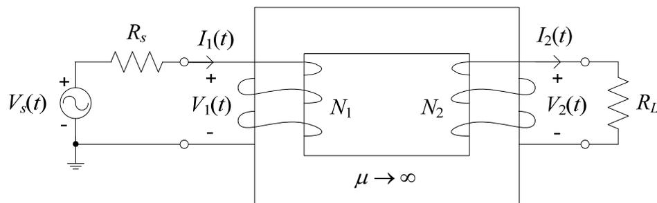
This transformer “transforms” the load resistance to the primary according to (12). An **equivalent circuit** at the primary terminal can be constructed using this **effective primary resistance**:
