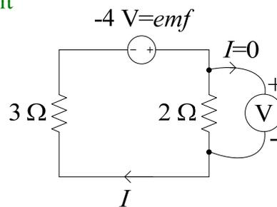
It is very important to note the **polarity of the equivalent emf voltage source** in this circuit. The contour  $c$  was initially chosen clockwise. Consequently, the current  $I$  must enter the '-' terminal of this voltage source, as shown.
