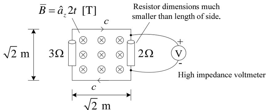
Interestingly, this circuit has no traditional source in it such as a voltage source or current source. So how can the voltmeter read anything but zero? The answer is by Faraday's law: an induced emf will cause a current to flow in the circuit!
