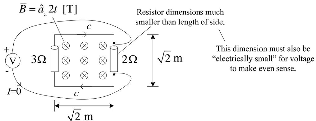
Our expectation might be that there won't be any change to the measured voltage. How could it since we've only changed how the leads of the high-impedance voltmeter are laid out. By Faraday's law and induced emf, however, we will see that there **is** a change to the measured voltage.
