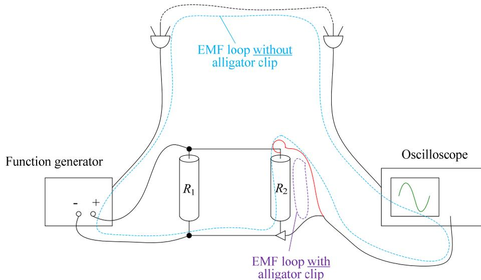
Measurements taken without connecting the scope probe alligator clip to ground will be correct at “low” frequencies (remember the scope is single-ended input).
