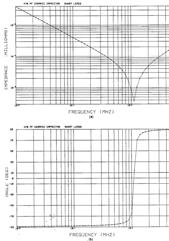
FIGURE 6.25 Measured impedance of a 470 pF ceramic capacitor with short lead lengths: (a) magnitude; (b) phase.
