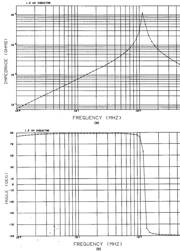
FIGURE 6.32 Measured impedance of a 1.2  $\mu\text{H}$  inductor having very short lead lengths: (a) magnitude; (b) phase.
