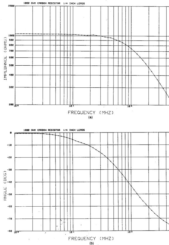
FIGURE 6.19 Measured impedance of a 1000  $\Omega$ , carbon resistor having ¼ inch lead lengths: (a) magnitude; (b) phase.
