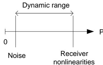
On the low end, the receiver is limited by noise. On the high end, the receiver is limited by the strongest signal it can receive without producing spurious responses.
