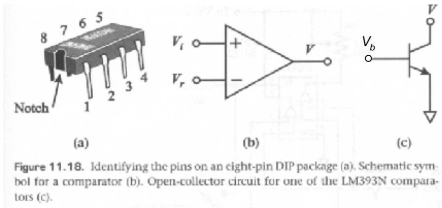
Figure 11.18. Identifying the pins on an eight-pin DIP package (a). Schematic symbol for a comparator (b). Open-collector circuit for one of the LM393N comparators (c).
