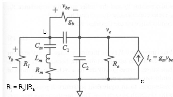
Figure 11.11. Equivalent circuit for the Clapp crystal oscillators.
