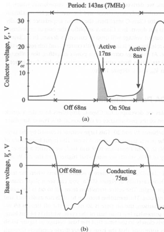
Figure 10.5. Voltages for the NorCal 40A Power Amplifier at 7 MHz. The output power is 2.5 W, with a supply voltage of 12.8 V and a supply current of 250 mA. The efficiency is 78%. Collector voltage (a), and base voltage (b).
