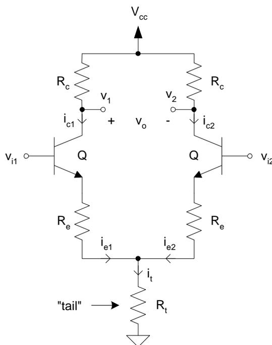
It's important that the circuit have **matched transistors and resistors** for satisfactory performance (more specifically, to ensure symmetry in the circuit).
