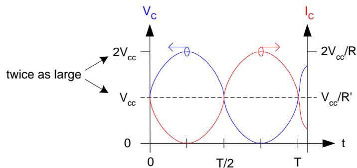
**Why** twice as large? Firstly, as just mentioned, the average value of the signal must equal  $V_{cc}$ . Then, on the negative swing the lowest voltage will be approximately  $0$  when  $Q$  is saturated. Hence, the signal amplitude at  $V_c$  is  $V_{cc}$ . Therefore, the maximum value is then  $V_{cc} + V_{cc} = 2V_{cc}$ .
