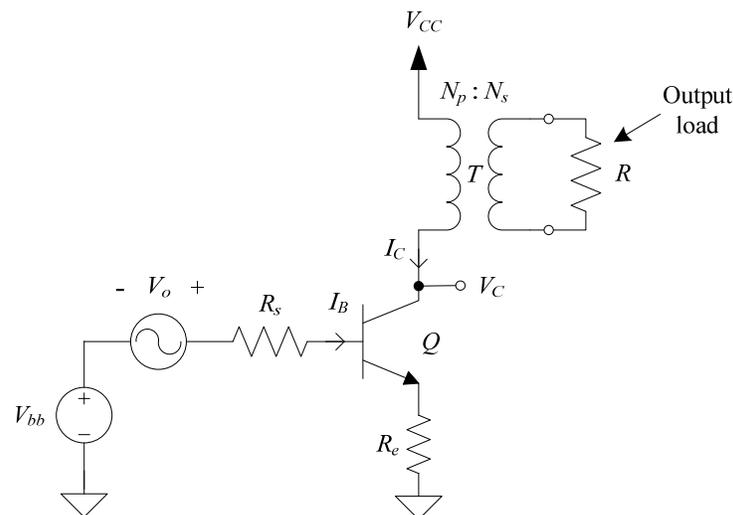
The Driver Amplifier (Q6) in the NorCal 40A is an example of such a class A amplifier with transformer load.
