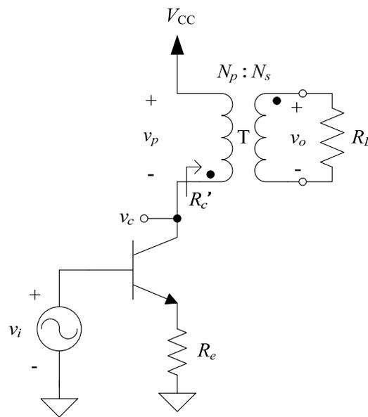
The expected voltage gain can be **calculated in two steps**. We'll assume that  $T$  is an ideal transformer, meaning we'll ignore the effects of the magnetization current in the transformer  $T$ . (Would that be a good assumption for the Driver Transformer  $T1$ ?)
