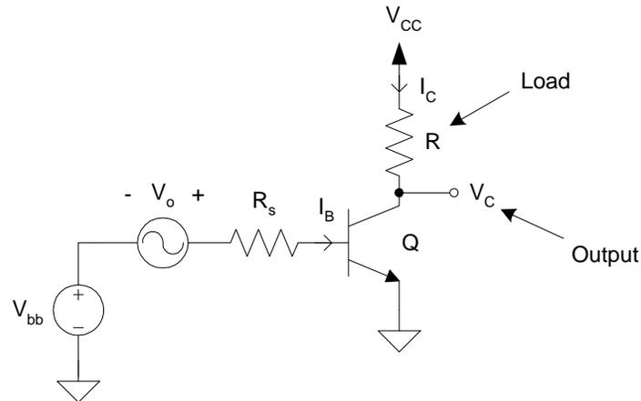
We will restrict ourselves for the time being to circuits of this type when  $Q$  remains entirely in the active region. Note that  $V_{bb}$  is the input bias (i.e., dc) voltage used to set this operational condition.
