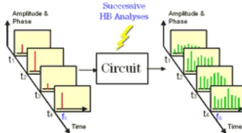
Harmonic Balance analysis is performed at each time step. This process creates a succession of spectra that characterize the response of the circuit at the different time steps.
