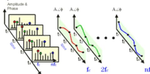
Circuit envelope provides a complete non steady-state solution of the circuit through a Fourier series with time-varying coefficients.
