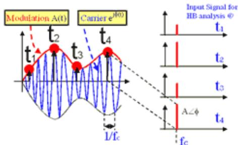
Each modulated signal can be represented as a carrier modulated by an envelope -  $A(t) \cdot e^{j\omega_0 t}$ . The values of amplitude and phase of the sampled envelope are used as input signals for Harmonic Balance analyses.
