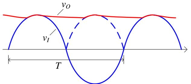
The “ripple frequency” is **twice** that of a half-cycle peak rectifier. Using the same derivation procedure as before with the half cycle, but with  $T \rightarrow T/2$  gives from (7)
