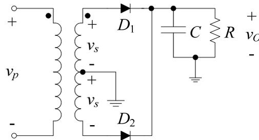
The output voltage has less ripple than from a half-cycle peak rectifier (actually **one half** less ripple).
