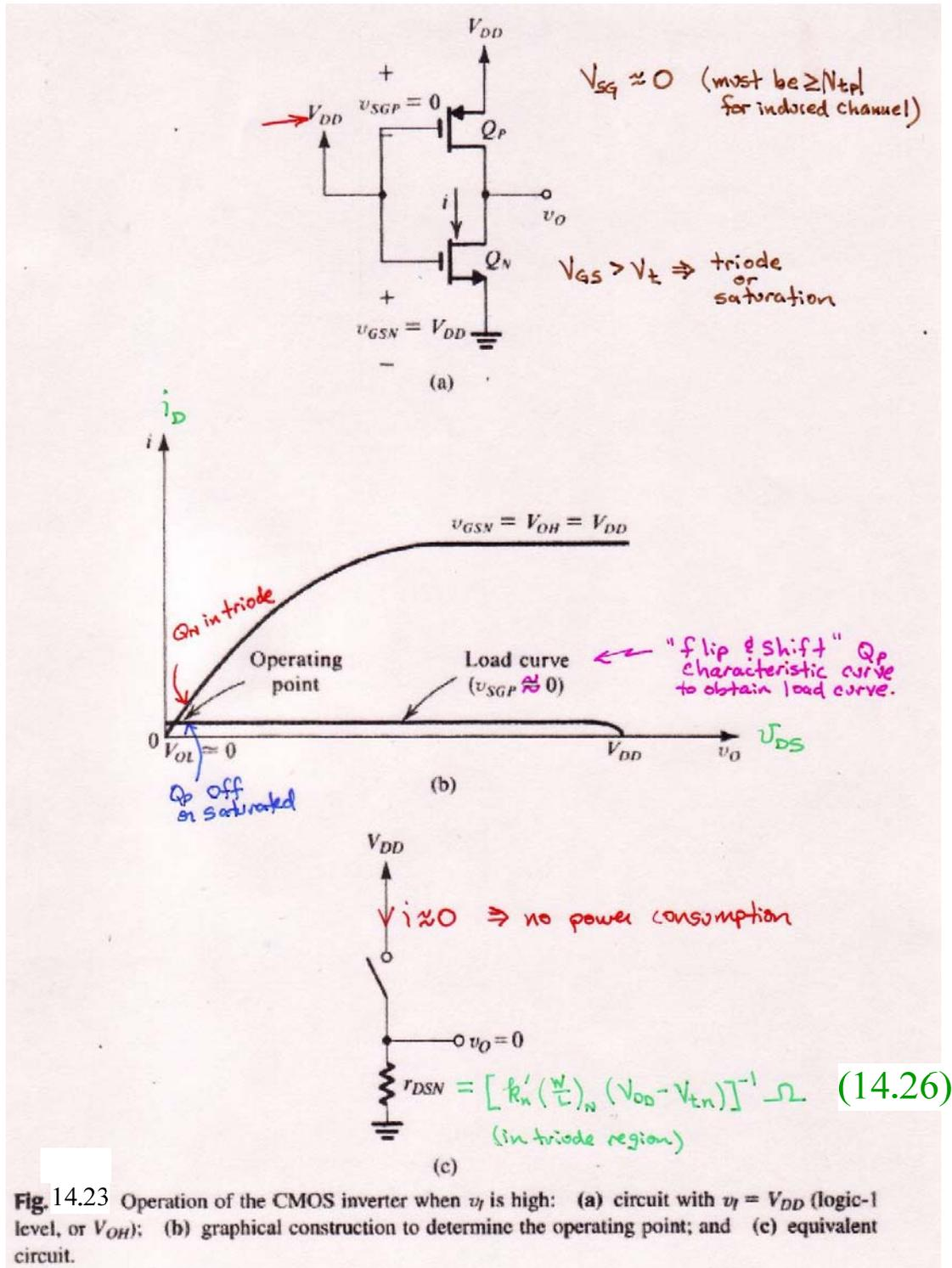
Fig. 14.23 Operation of the CMOS inverter when  $v_I$  is high: (a) circuit with  $v_I = V_{DD}$  (logic-1 level, or  $V_{OH}$ ); (b) graphical construction to determine the operating point; and (c) equivalent circuit.
