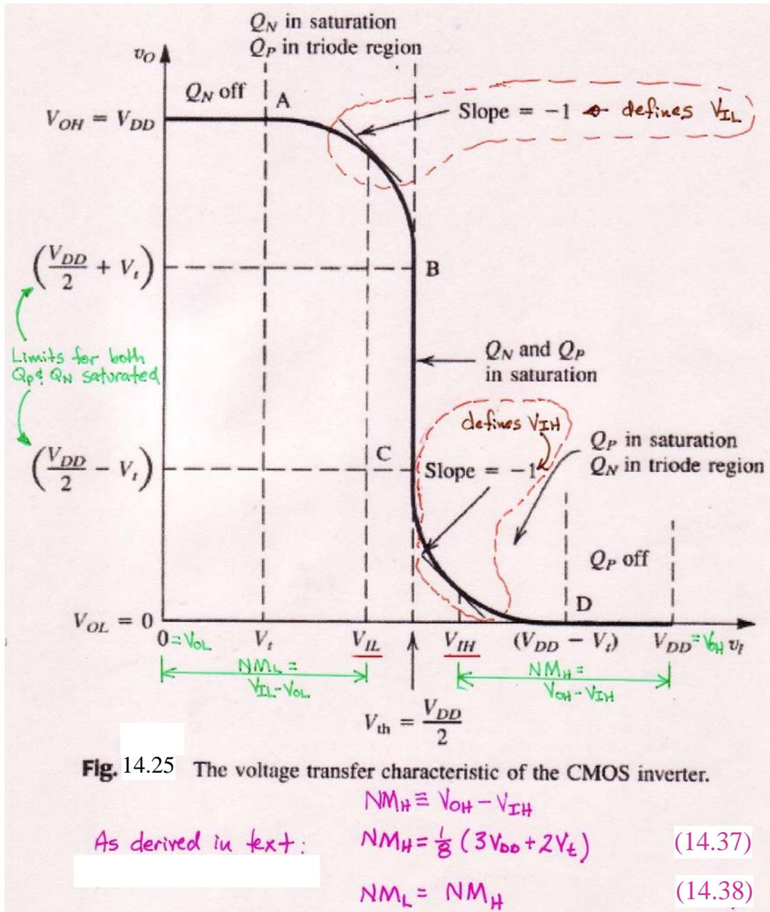
Note that the use of MOSFETs for a digital circuit such as this inverter in Fig. 14.25 is using the extremes of the VTC. This is very different than when MOSFETs are used as small signal amplifiers where the linear region of the VTC is used.
