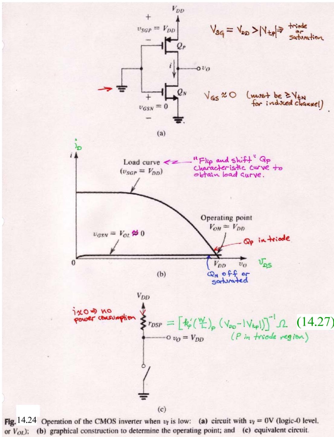
**Fig. 14.24** Operation of the CMOS inverter when  $v_I$  is low: (a) circuit with  $v_I = 0$  V (logic-0 level, or  $V_{OL}$ ); (b) graphical construction to determine the operating point; and (c) equivalent circuit.
