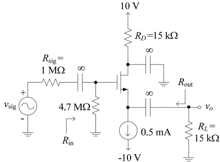
Notice the addition of the **bypass capacitor** on the drain terminal of the MOSFET. This was added so that  $R_D$  will affect only the DC functionality of the circuit. In the AC operation, the drain terminal will be an AC ground, which fits the analysis presented in this lecture.
